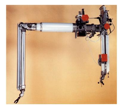
Fig.1. MT200 Mechanical Master Slave System
