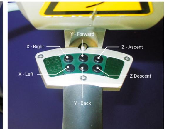
Electrical control buttons for MT 200 remote manipulator
