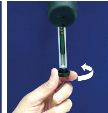
Counter clockwise = Tongs closing
