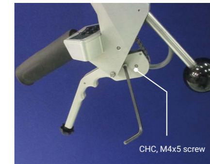
Adjustment of the handle opening
